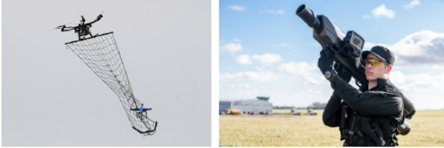
IMAGE 28. METHODS OF CAPTURING DRONES WITH NETS
